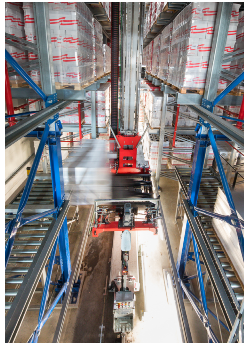
AUTOMATICO CON SATELLITE E TRASLOELEVATORE AUTOMATED STORAGE & RETRIEVAL SYSTEM WITH SHUTTLE AND STACKER CRANE
